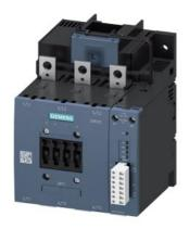
power contactor, AC-3 185 A, 90 kW / 400 V AC (50-60 Hz) / DC operation 96-127 V AC/DC auxiliary contacts 1 NO + 1 NC 3-pole, frame size S6 busbar connections drive: electronic with PLC / SIMOCODE - interface and remaining lifetime signal
