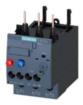
Overload relay 30...36 A Thermal For motor protection Size S0, Class 10 Contactor mounting Main circuit: Screw Auxiliary circuit: Screw Manual-Automatic-Reset
