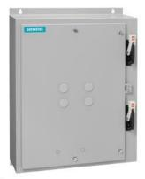
Duplex starter w/o alternator, Size 1, Three phase full voltage, Solid-state overload relay, OLR amp range 0.75-3.4A, 190-220/220-240V 50/60Hz coil, Combination type, Two 3A circuit breakers, Enc NEMA type 4 painted steel, Water/dust tight for outdoors
