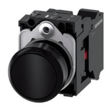
Pushbutton, 22 mm, round, plastic, black, pushbutton, flat, momentary contact type, with holder 1 NC, spring-type terminal, with laser labeling, upper case
