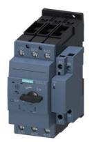
Circuit breaker size S2 for motor protection, CLASS 10 with overload relay function A-release 22...32 A N-release 416 A screw terminal Standard switching capacity
