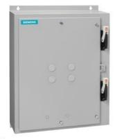
Duplex starter w/ alternator, Size 1, Three phase full voltage, Solid-state overload relay, OLR amp range 5.5-22A, 110V 50Hz / 120V 60Hz coil, Combination type, Two 25A circuit breakers, Enclosure NEMA type 12, Dust/drip proof for indoors
