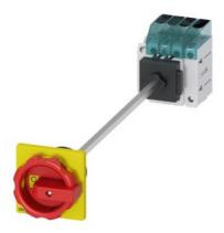
Load disconnector 3LD3, lu 40 A Main switch 3-pole + N Rated operating capacity at AC-23 A at 400 V 18.5 kW floor mounting Basic switch with door coupling Central hole mounting 22.5mm Rotary actuator red / yellow 66 x 66 mm with auxiliary switch 1OE + 1S
