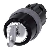
RONIS key-operated switch, 22 mm, round, plastic with metal front ring, lock number SB30, with 2 keys, 3 switch positions I-O<II, left latching, right momentary contact type, actuating angle 2x45°, 10:30h/12h/13:30h, key removal O, possible special locks: SB31, 421, 455, with laser labeling, upper case and lower case, always upper case at the beginning of the word
