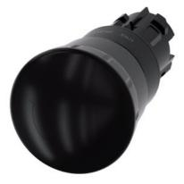
Mushroom pushbutton, 22 mm, round, plastic, black, 40 mm, positive latching, acc. to EN ISO 13850, rotate-to-unlatch, with laser labeling, upper case and lower case, always upper case at beginning of line
