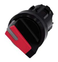
Selector switch, illuminable, 22 mm, round, plastic, red, selector switch, short, 2 switch positions O<I, momentary contact type, Actuating angle 45°, 10:30h/12h, with laser labeling, inscription or symbol Customer-specific selection with SIRIUS ACT configurator (CIN)
