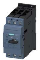
Circuit breaker size S2 for motor protection, Class 20 A-release 35...45 A N-release 650 A screw terminal Standard switching capacity
