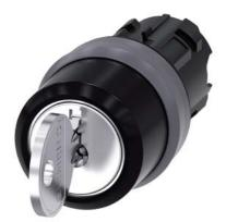
RONIS key-operated switch, 22 mm, round, plastic with metal front ring, lock number SB30, with 2 keys, 3 switch positions I-O<II, left latching, right momentary contact type, actuating angle 2x45°, 10:30h/12h/13:30h, key removal O, possible special locks: SB31, 421, 455, with laser labeling, lower case
