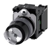
RONIS key-operated switch, 22 mm, round, plastic with metal front ring, lock number SB30, with 2 keys, 2 switch positions O-I, latching, actuating angle 90°, 10:30h/13:30h, key removal O+I, with holder, 1 NO, screw terminal, possible special locks: SB31, 421, 455, with laser labeling, lower case
