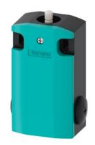
Basic switch for position switch 3SE5162 Metal enclosure XL, 56 mm wide Device connection  $3x(M20\ x\ 1.5)$  IP66/IP67 2 x (1 NO/2 NC) Slow-action contacts without actuator head
