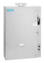
Pump control panel, Size 3, Three phase full voltage, Solid-state overload relay, OLR amp range 25-100A, 110V 50Hz / 120V 60Hz coil, Standard type contactor, 200A fusible disconnect, 200A/600V fuse clip, HOA Sel Sw. <(>&<)> Start P.B., Enclosure NEMA type 3/3R, Weather proof outdoor use
