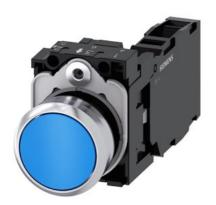
Pushbutton, 22 mm, round, metal, shiny, blue, pushbutton, flat, momentary contact type, 1 NO+1 NC, screw terminal, Z=20-unit packaging
