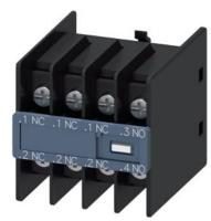
Auxiliary switch on the front, 1 NO + 3 NC Current path 1 NC, 1 NC, 1 NC, 1 NO, 1 NO for 3RH and 3RT Ring cable lug connection .1/.2, .1/.2, .1/.2, .3/.4
