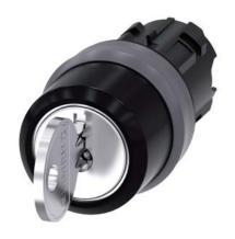
RONIS key-operated switch, 22 mm, round, plastic with metal front ring, lock number SB30, with 2 keys, 3 switch positions I>O<II, momentary contact type, actuating angle 2x45°, 10:30h/12h/13:30h, key removal O, possible special locks: SB31, 421, 455, with laser labeling, lower case
