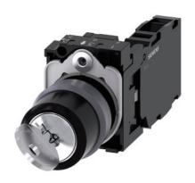
RONIS key-operated switch, 22 mm, round, plastic with metal front ring, lock number SB30, with 2 keys, 2 switch positions O-I, latching, actuating angle 90°, 10:30h/13:30h, key removal O+I, with holder, 1 NO+1 NC, screw terminal, possible special locks: SB31, 421, 455, with laser labeling, upper case
