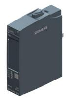
SIMATIC ET 200SP, Digital input module, DI 8x 24V DC Basic, type 2 (IEC 61131), sink input, (PNP, P-reading), Packing unit: 10 pieces, fits to BUtype A0, Colour Code CC01, input delay time 0,05..20ms, module diagnostics for: supply voltage
