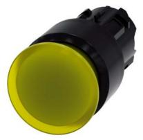
Illuminated mushroom pushbutton, 22 mm, round, plastic, yellow, 30 mm, latching, pull-to-unlatch mechanism, with laser labeling, lower case
