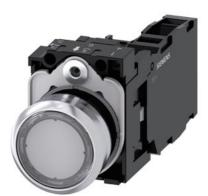
Illuminated pushbutton, 22 mm, round, metal, shiny, clear, pushbutton, flat, momentary contact type, with holder, 1 NO+1 NC, LED module with integrated LED 110 V AC, screw terminal, with laser labeling, lower case
