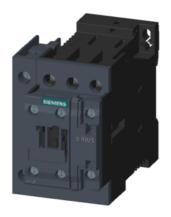
Contactor, AC-1, 40 A/400 V/40  $^{\circ}\text{C},$  S0, 4-pole, 220 V DC, 1 NO+1 NC, screw terminal
