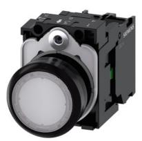
Illuminated pushbutton, 22 mm, round, plastic, white, pushbutton, flat, momentary contact type, with holder, 1NO, LED module with integrated LED 230 V AC, screw terminal, with laser labeling, upper case
