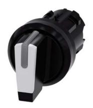
Selector switch, illuminable, 22 mm, round, plastic, white, selector switch, short, 3 switch positions I-O<II, left latching, right momentary contact type, actuating angle  $2x45^{\circ}$ , 10:30h/12h/13:30h
