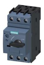
Special type Circuit breaker size S00 for motor protection, CLASS 10 A-release 4.5...6.3 A N-release 82 A screw terminal Standard switching capacity Ambient temperature -50  $^\circ$ C 500 switching cycles
