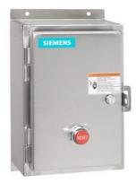
Non-reversing motor starter, Size 1, Three phase full voltage, Solid-state overload relay, OLR amp range 3-12A, Non-combination type, Encl. type 4X 304 S. Steel, Water/dust tight noncorrosive, Standard width enclosure
