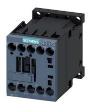
Power contactor, AC-3 16 A, 7.5 kW / 400 V 1 NC, 24 V DC communication-capable, 3-pole Size S00, screw terminals
