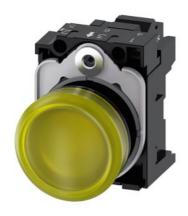
Indicator lights, 22 mm, round, plastic, yellow, lens, smooth, with holder, LED module with integrated LED 110 V AC, spring-type terminal, with laser labeling, upper case
