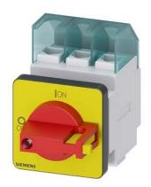
SENTRON, Switch disconnector 3LD, emergency switching-off switch, 3-pole, lu: 25 A, operating power / at AC-23 A 400 V: 9.5 kW, floor mounting with door coupling, knob-operated mechanism, red/yellow, 4-hole mounting of the handle
