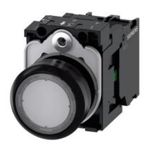
Illuminated pushbutton, 22 mm, round, plastic, clear, pushbutton, flat, momentary contact type, with holder, 1NO, LED module with integrated LED 110 V AC, screw terminal, with laser labeling, upper case and lower case, always upper case at beginning of line
