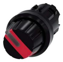
Selector switch, illuminable, 22 mm, round, plastic, red, Rotary knob, 2 switch positions O-I, latching, actuating angle  $90^{\circ}$ , 10:30h/13:30h Z=50-unit packaging
