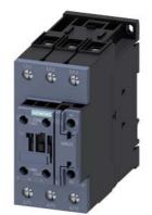
power contactor, AC-3 51 A, 22 kW / 400 V 1 NO + 1 NC, 24 V AC, 50 Hz, 3-pole, size S2, screw terminal
