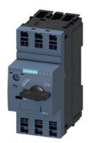
Special type Circuit breaker size S00 for motor protection, CLASS 10 A-release 1.1...1.6 A N-release 21 A Spring-type terminal Standard switching capacity Ambient temperature -50  $^\circ$ C 500 switching cycles
