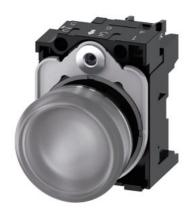
Indicator lights, 22 mm, round, metal, shiny, clear, lens, smooth, with holder, LED module with integrated LED 110 V AC, screw terminal, Z=20-unit packaging
