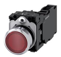
Illuminated pushbutton, 22 mm, round, metal, shiny, red, pushbutton, flat, momentary contact type, with holder, 1 NO+1 NC, LED module with integrated LED 110 V AC, screw terminal, with laser labeling, upper case and lower case, Always upper case at the beginning of the word
