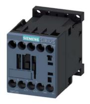
power contactor, AC-3 9 A, 4 kW / 400 V 1 NO, 24 V DC 0.7-1.25\* US, with diode integrated, 3-pole, size S00, screw terminal suitable for PLC outputs not expandable with auxiliary switch
