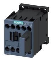
power contactor, AC-3 12 A, 5.5 kW / 400 V 1 NO, 24 V DC 0.7-1.25\* US, with varistor plugged on, 3-pole size S00, screw terminal not expandable with auxiliary switch
