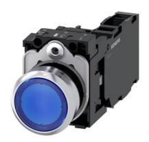
Illuminated pushbutton, 22 mm, round, metal, shiny, blue, pushbutton, flat, momentary contact type, with holder, 1 NO+1 NC, LED module with integrated LED 110 V AC, screw terminal, with laser labeling, symbol number according to, ISO 7000 or IEC 60417
