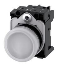
Indicator lights, 22 mm, round, plastic, white, lens, smooth, with holder, LED module with integrated LED 110 V AC, screw terminal, with laser labeling, upper case
