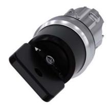
Key-operated switch O.M.R, 22 mm, round, metal, shiny, lock number 73034, black, with 2 keys, 2 switch positions O<I, momentary contact type, Actuating angle  $45^{\circ}$ , 10:30h/12h, key removal O, Z=50-unit packaging
