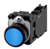
Pushbutton, 22 mm, round, plastic, blue, pushbutton, flat, momentary contact type, with holder 1 NO+1 NC, spring-type terminal, Z=20-unit packaging
