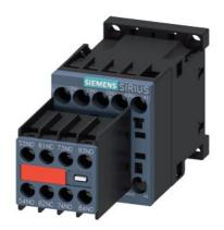
contactor relay, 7 NO + 1 NC, 110 V AC, 50 Hz / 120 V, 60 Hz, size S00, screw terminal, captive auxiliary switch
