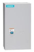
Reversing motor starter, Size 3, Three phase full voltage, Solid-state overload relay, OLR amp range 25-100A, 110V 50Hz / 120V 60Hz coil, Non-combination type, Enclosure type 1, Indoor general purpose use, Standard width enclosure
