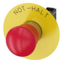
EMERGENCY STOP mushroom-type actuator, 22 mm, round, metal, shiny, red, 40 mm, positive latching, according to EN ISO 13850, rotate-tounlatch, with yellow backing plate, inscription: NOT-HALT, with holder, 1 NC, spring-type terminal, Z=20-unit packaging
