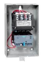
Non-reversing motor starter, Size 00, Three phase full voltage, Solid-state overload relay, OLR amp range 0.75-3.4A, Non-combination type, Enclosure type 1, Indoor general purpose use, Extra-wide enclosure
