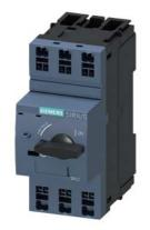
Circuit breaker size S00 for starter combination Rated current 10 A N release 130 A Spring-type terminal Standard switching capacity
