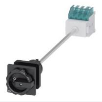
SENTRON, Switch disconnector 3LD, main switch, 3-pole, lu: 16 A, Operating power / at AC-23 A at 400 V: 7.5 kW, floor mounting with door coupling, rotary operating mechanism, black, central mounting 22.5 mm of the handle
