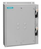
Duplex starter w/o alternator, Size 1, Three phase full voltage, Solid-state overload relay, OLR amp range 0.25-1A, 190-220/220-240V 50/60Hz coil, Combination type, Two 3A circuit breakers, Encl NEMA type 4X 304 S-Steel, Water/dust tight noncorrosive
