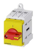
Load disconnector 3LD3, lu 63 A Main switch 3-pole Rated operating capacity at AC-23 A at 400V 22.0 kW Installation in distribution boards, Basic switch with selector knob red / yellow
